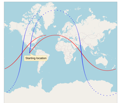
Fig. 28: The ground track over 120 minutes of two satellites orbiting at inclinations of 50^\circ and 80^\circ .
